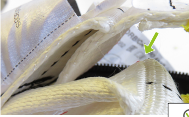
• No tearing of the energy absorber
