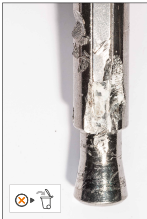
• Marked shaft, broken wedge plate
